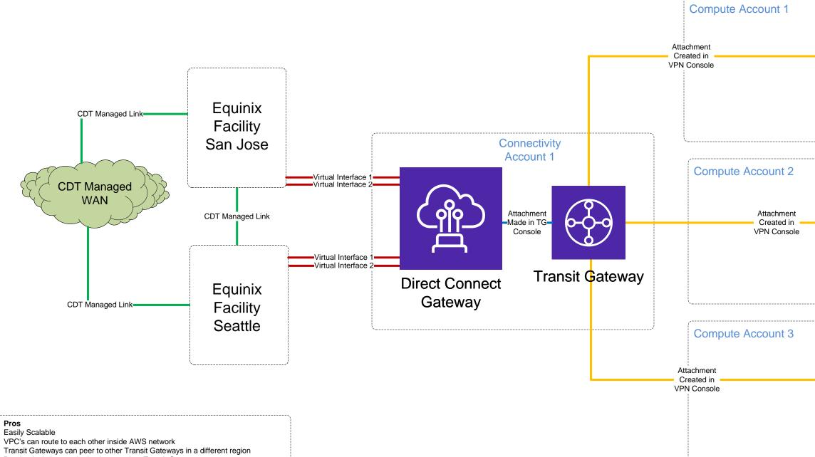
Routing Isolation can be implemented on Transit Gateways in a diffe Geographic Redundancy for CPI Connectivity
