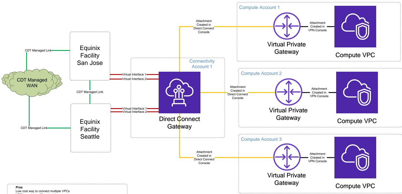
VPC's can be in different regions VPC's can be in different accounts Geographic Redundancy for CPI Connectivity
