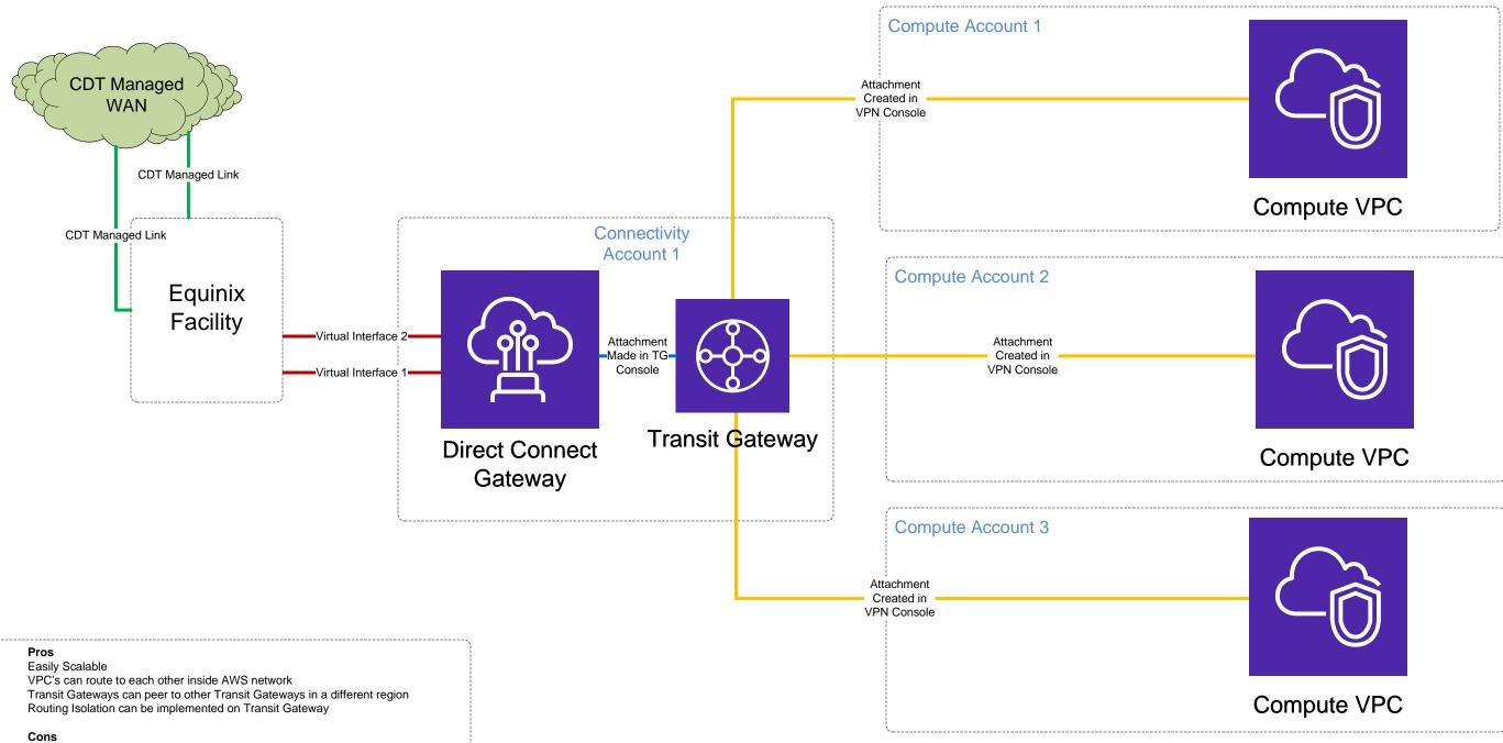
Dedicated hand off needed, with additional cost Additional AWS costs for data transfer on transit gateway VPCs can not be put in different VRF's on prem VPCs must be in the same region as the transit gateway they attach to
